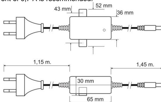
Fig.1. Dimension of power supply.
